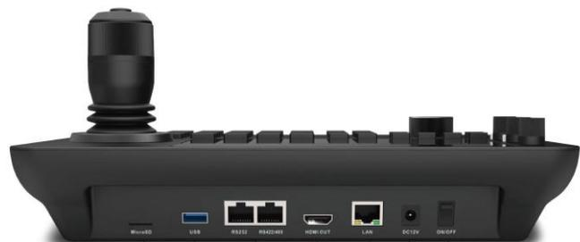
Micro SD/TF Card Slot    USB Port    RS485/RS422/RS232    HDMI Output    Network Interface    Power Connector    Power Switch
